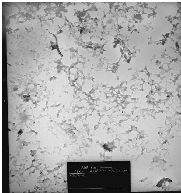
Fig. 1 – Transmission Electron Microscopy of PMMA/CNT nanocomposites
