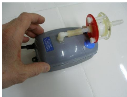
Fig. 3 – A simple collector of aerosol and NA based on use of a water-soluble nanofilter
