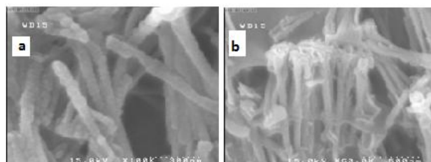
Fig. 4 – a) SEM image of nanowires with 35 nm diameters and 2.1 mm length and (b) with 20 nm diameter and 2.5 mm length
