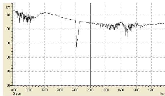
Fig. 6 – FTIR results for Graphene-PANI nanocomposites
