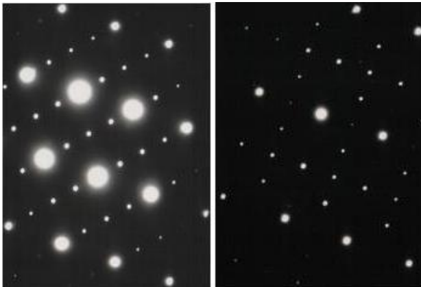
Fig. 3 – Two electron diffraction patterns taken from the CuZnAl and CuAlMn alloy samples
