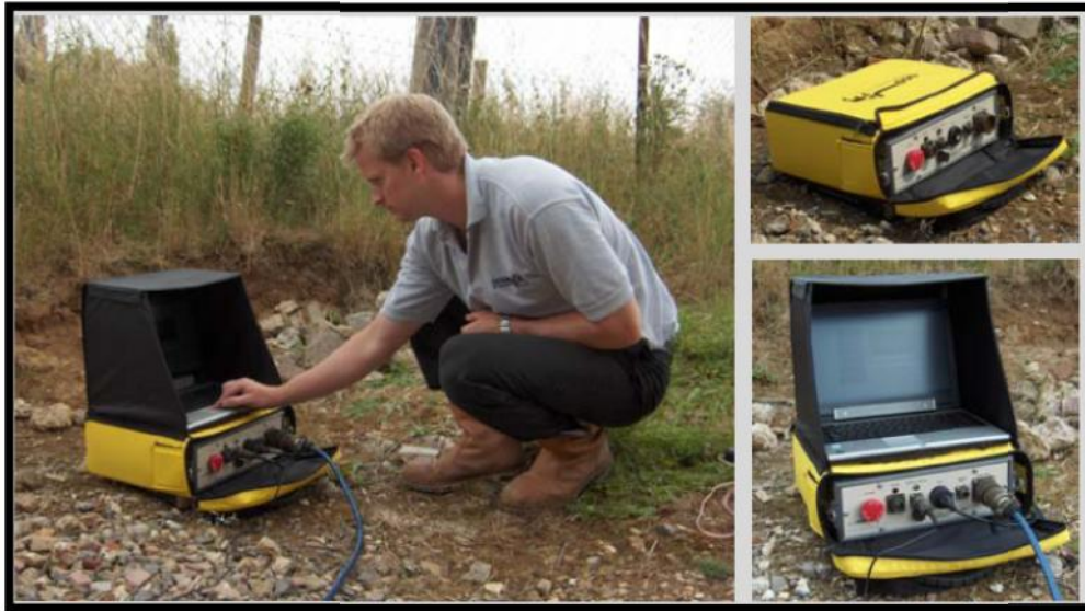
Figure 2.4: Testing SASW kit on soil. Source; ( http:// www.gdsinstruments.com )
