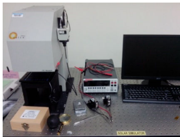
Fig 2.9: I-V characteristic measurement with solar simulator taken from MiNT-SRC, UTHM
