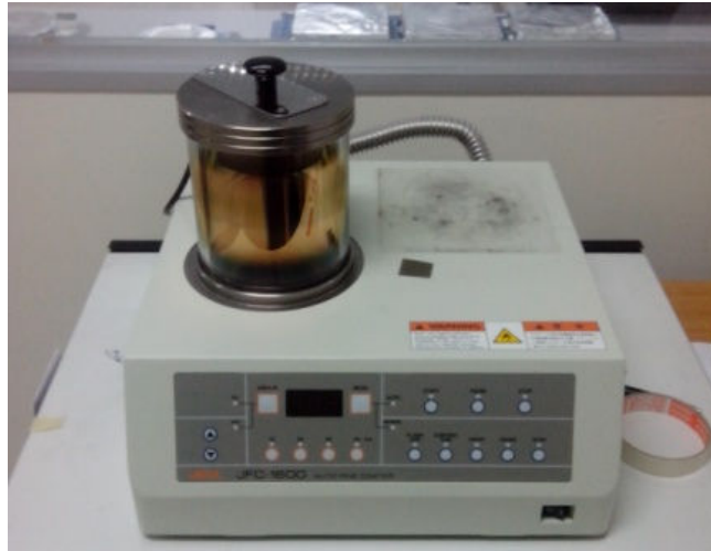
Fig. 2.5: Sputter coater gold/platinum to coat metal electrode of organic solar cell
