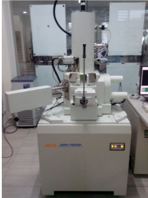
Fig.2.6: FESEM/EDS to characterize LiF composite and size
