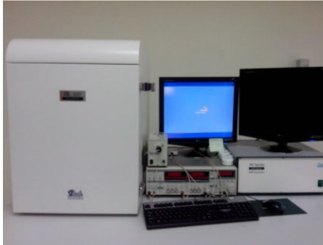
Fig. 2.7: Atomic Force Microscope (AFM) to characterize surface roughness of LiF compare to glass substrate
