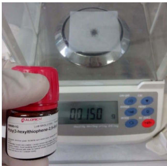
Fig.3.2: 15mg [6,6] - phenyl-C 61 butyric acid methyl ester (PCBM)
