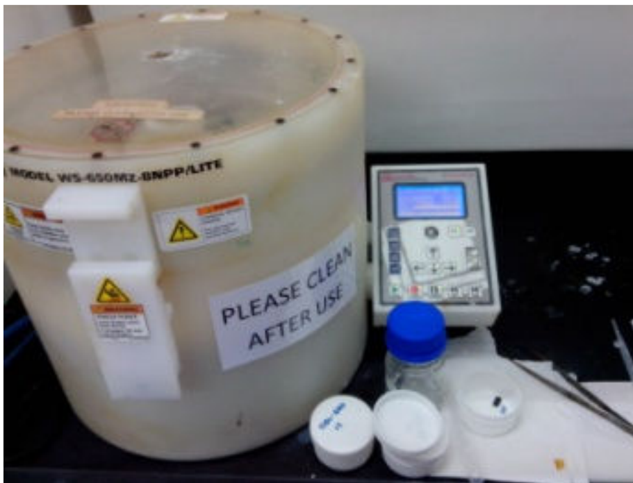
Fig.2.1: Spin coater machine to coat LiF layer on glass or active layer substrate
