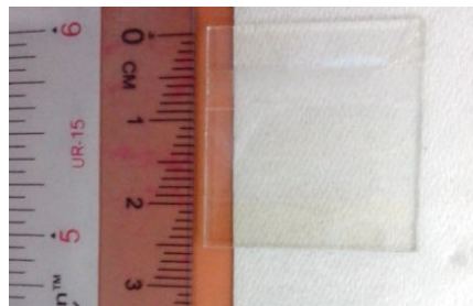
Fig.3.5: ITO etched on glass substrate 2.5cm X 2.5cm dimension
