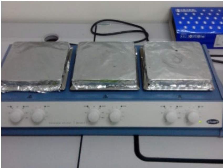
Fig.2.2: Magnetic stirrer machine to dilute LiF and active layer solution
