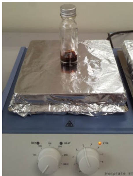
Fig.3.4: Ageing process of P3HT: PCBM
