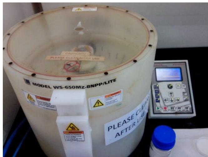
Fig.3.7: Spin-Coater Machine is used to coated active layer and LiF solution on glass substrate
