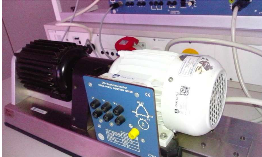
Figure 2.1: The three phase induction motor
