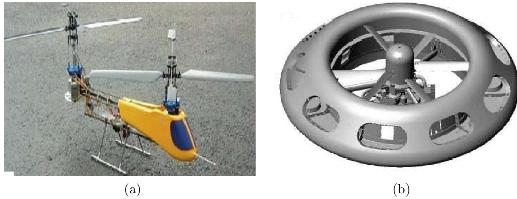
Figure 2.12: Tandem and ducted twin-rotor helicopter: (a) Tandem, and (b) Ducted twin-rotor UAV (Tech-Model-Product, 2010; Avanzini et al. , 2005)
