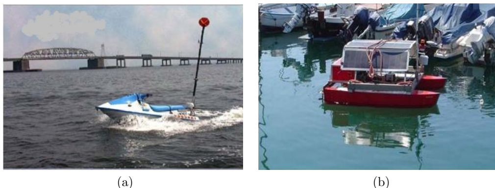
Figure 2.6: Single-mode USVs on the water surface operation: (a) X-Class USV, and (b) Charlie USV (Thomsen et al. , 2007; Caccia et al. , 2008)
