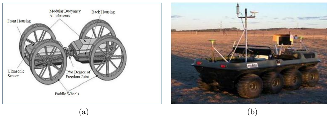
Figure 2.8: Unmanned autonomous amphibious vehicle: (a) Autonomous amphibious vehicle, and (b) ARGO (Michael & Nokleby, 2008; Tran et al. , 2004)
