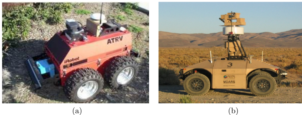
Figure 2.5: Single-mode UGVs on the ground locomotion: (a) ATRV, and (b) MDARS (DelFly, 2012; Pornsin-Sirirak et al. , 2001)
