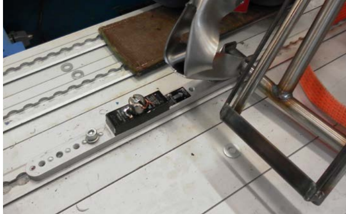
Fig 75. - The deformed channelling of the skate that remained in the tracking
