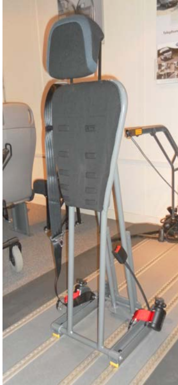
Fig 82. – The Artemis fitted into tracks
