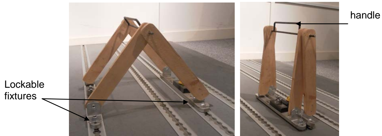
Fig 60. - Scissor action folding mechanism
