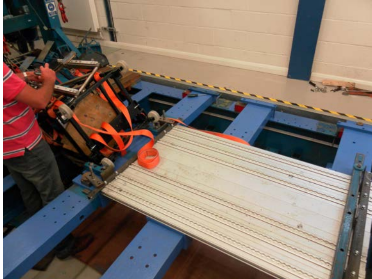
Fig 72. - Showing the back restraint and wheelchair pulled out of the floor
