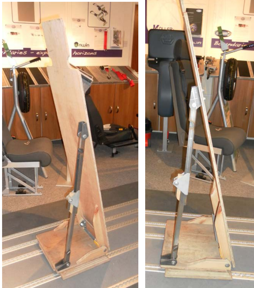
Fig 45. - Mock up of the composite model with mechanical fixing and lock down mechanism in place
