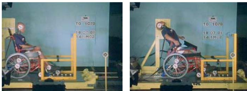
Fig 17. - Test 1 Wheelchair occupant during sled test in manual wheelchair with no extra back or head restraint. (19)
