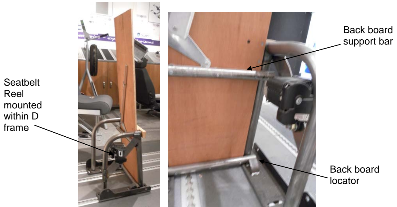
Fig 58. - The back board fitted into the base unit
