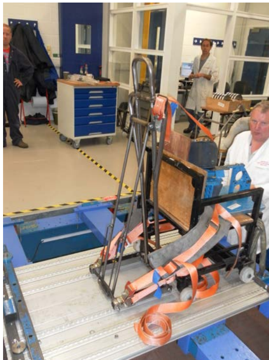
Fig 79. - Back restraint and wheelchair after passed test
