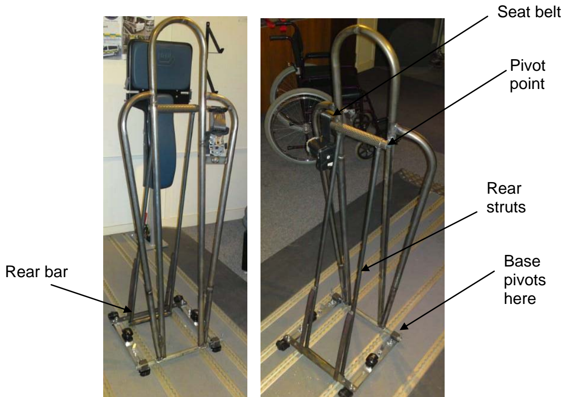
Fig 61. – Concept 7 (Front Pivot design)
