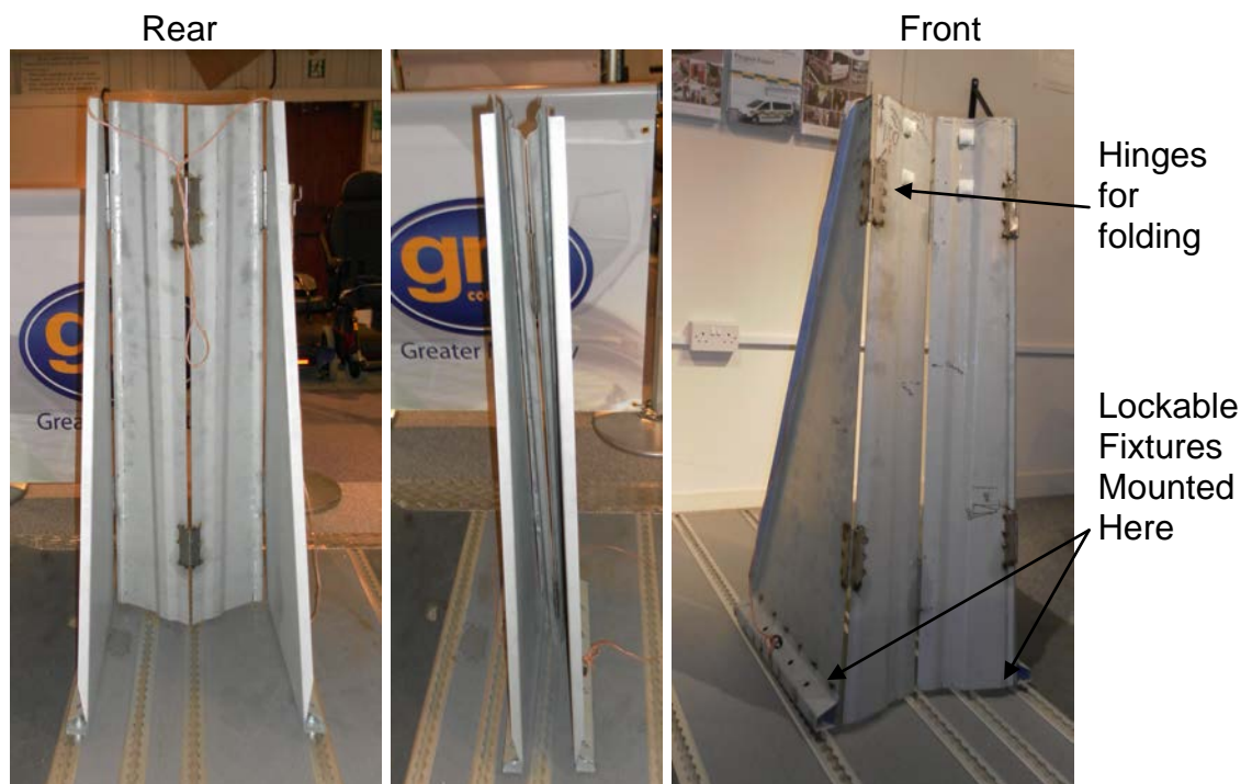
Fig 40. – Concept 2 (Folded Sheet Aluminium Back Restraint)
