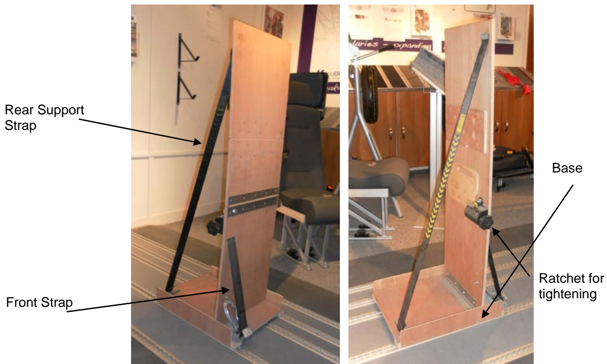
Fig 46. – Concept 5 (Webbing folding design) in its deployed position
