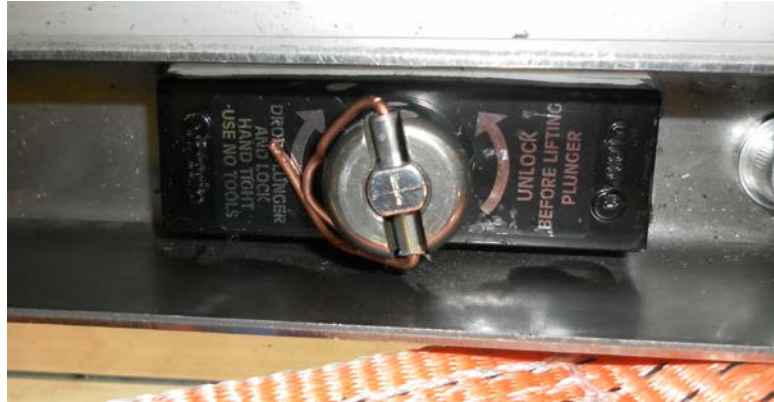
Fig 73. - Image showing the turning pin located to raise the locking pin to its original position
