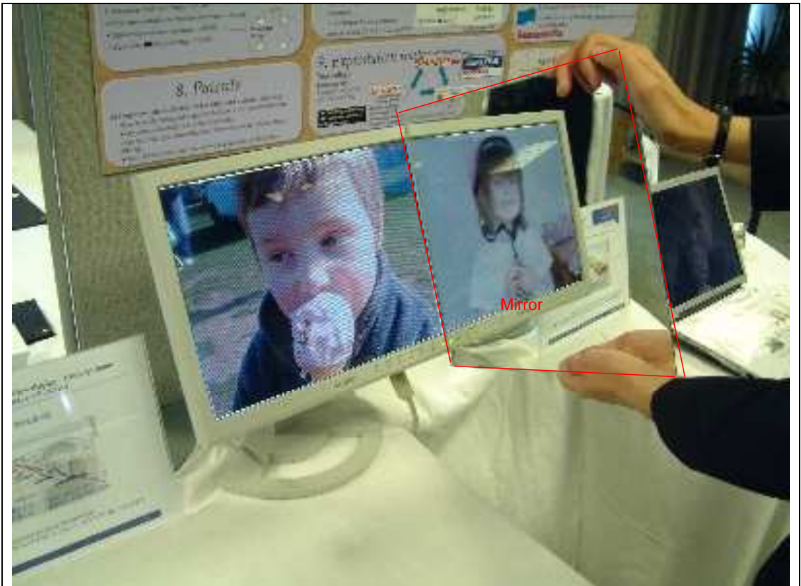
Figure 25: A photo of an early dual view prototype display. A mirror is used to show that a different image is being shown in another direction.
