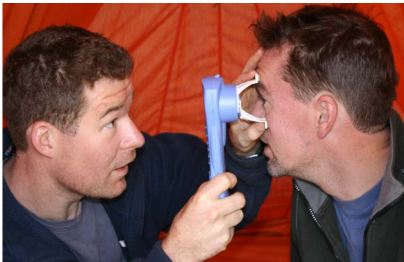
Figure 2-11 ForSite Digital Pupilometer (Neuroptics Inc, Irvine CA) being used without light excluding black cover.
