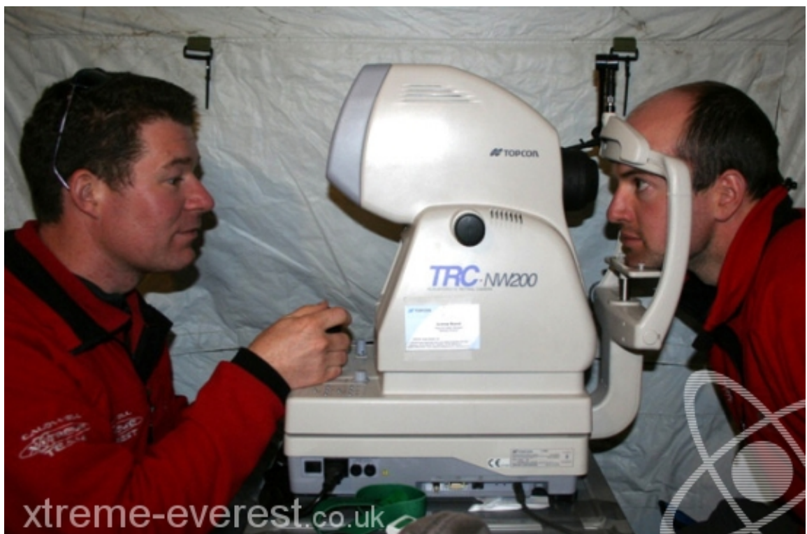
Figure 2-7 The TopCon 8MegaPixel Non-Dilating retinal camera in use in the research tent at Everest Base Camp (5300m).
