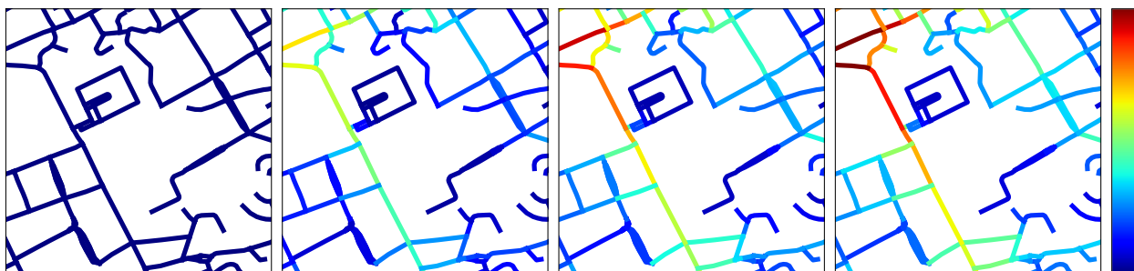
Figure 9 The evolution of the system when one link is removed from the network. The removal is as demonstrated in Figure 8, and betweenness values are recalculated accordingly. As previously, segments have been coloured according to the value of Q . The parameter values are \eta = 0.4 , \Gamma = 0.5 and \omega = 0.7 , and the value of \delta t used in the simulations is 0.01.
