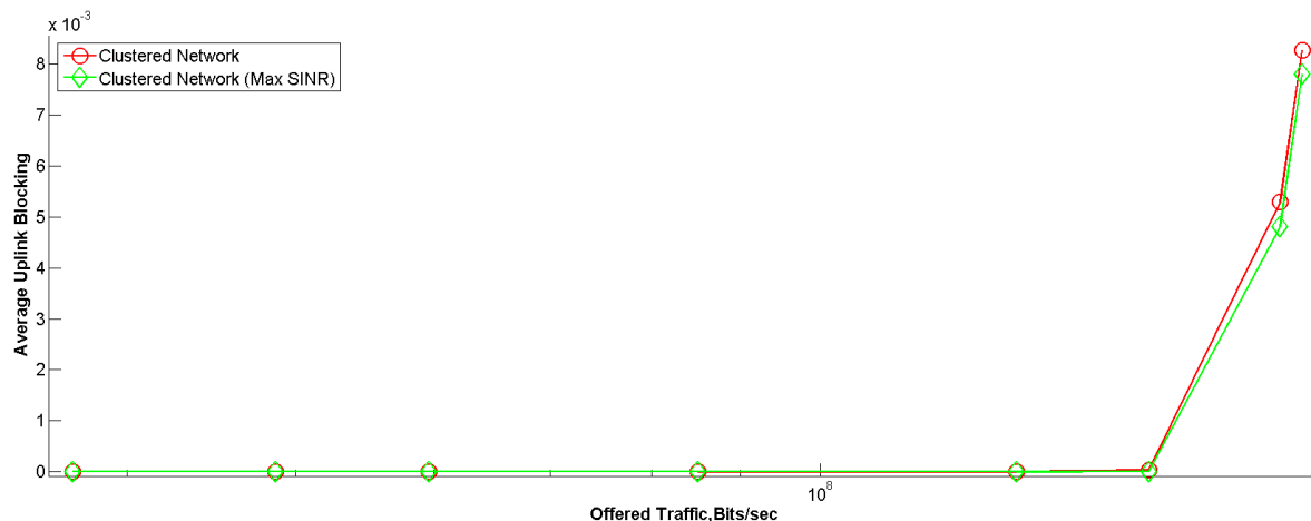
Figure 5-11: The blocking probability suffered at the uplink by dual hop clustered networks for various offered traffic levels.
