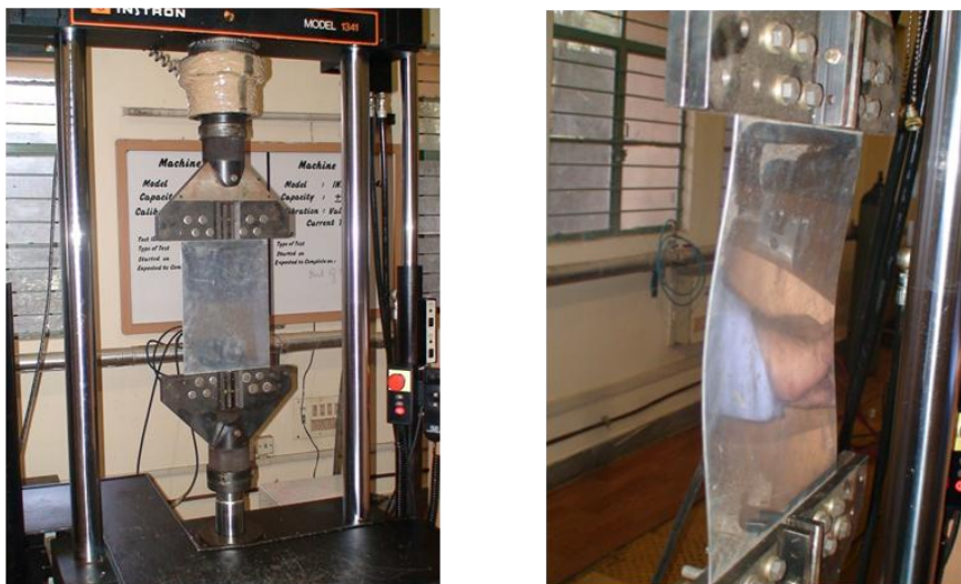
Figure 1: Buckling test setup and onset of buckling in rectangular aluminum plate
