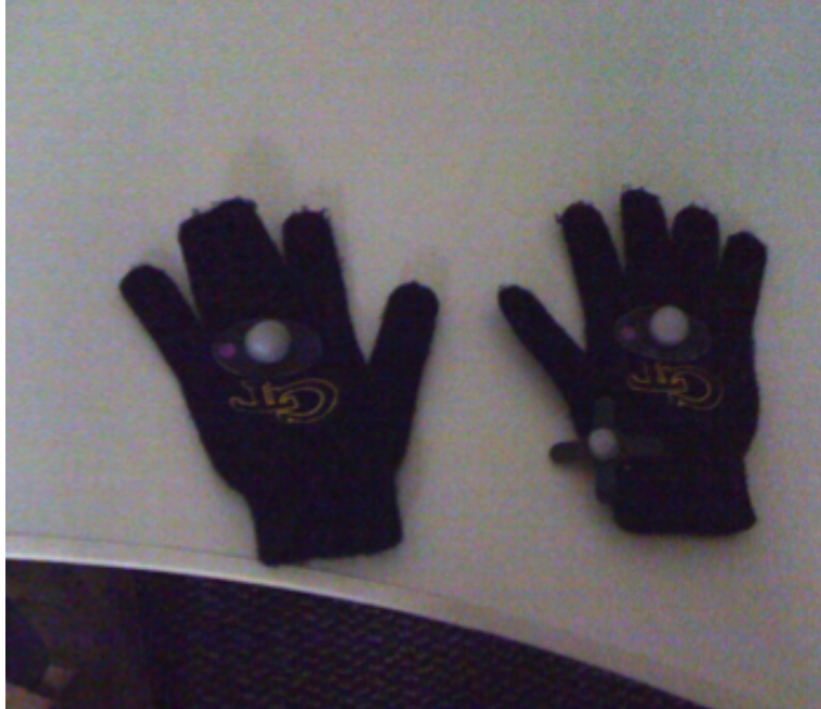
Figure 3: Optical markers (white spheres) used for collecting motion capture data fastened to gloves worn by the subject while performing the activities.
