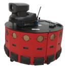
Figure 27: Shown is a picture of the IRobot Magellan-pro.
