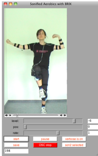
Figure 3: Screenshot of the GUI in sc3: The interface allows the playback of data synchronous to the recorded video, allowing playback control (via the rate slider) and real-time adjustment of the mapping functions. This accelerates and facilitates the optimization of the sonification.
