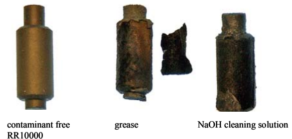
Figure 17. Appearance of samples exposed after 200 hours in air – 300 vpm SO 2 at 700°C (screening test).
