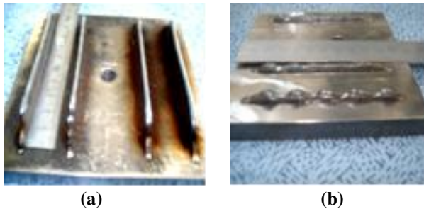
Fig. 5(a): Trial sample 7a with no hump and (5b): trial sample 7b exhibiting humping defects.
