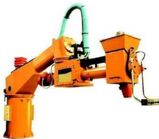
Figure 4-6 Typical structure of a continuous mixer , containing a muller wheel and plough blade (A-Yite-group-Limited, 2012)
