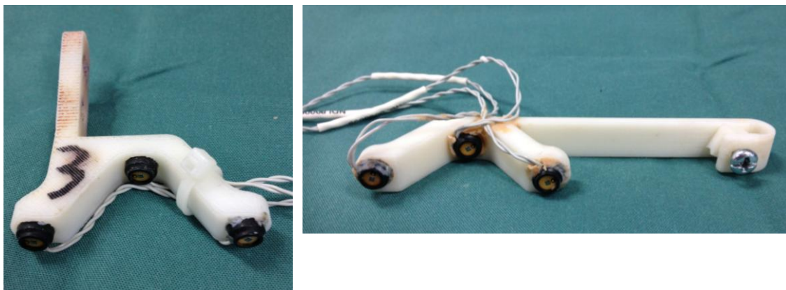
Figure 3.14. Optotrak rigid body markers (3x LEDs) for attachment to the spinous processes (left) and each of the semi-constrained or a single rigid rod component (right).
