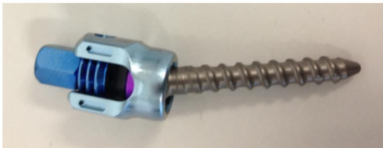
Figure 3.2. Medtronic 4.5 x 25mm CD Horizon ® Legacy™ multi-axial screws with break-off set screw not yet broken off.
