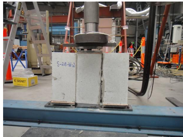
(b) Triplet failure (bond Failure)
