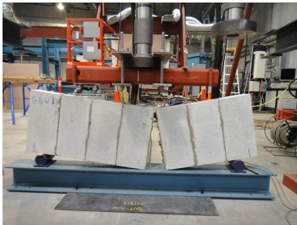
(a) Beam failure (bond failure)
