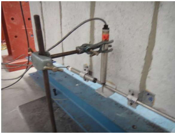
(a) LVDT positions on beam
