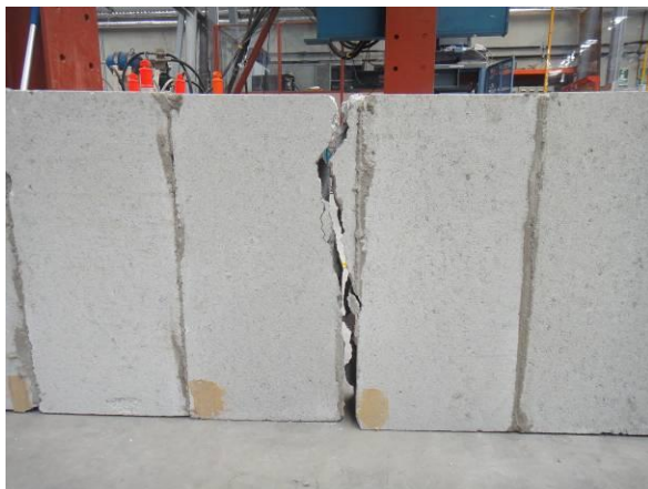
(c) Beam (partial block failure)
