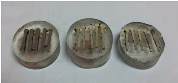
Fig. 7 : Photographs of prepared specimen for metallographic examination
