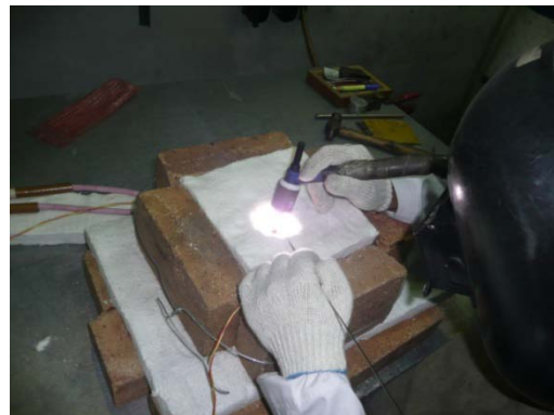
Fig. 5 : GTAW process being performed
