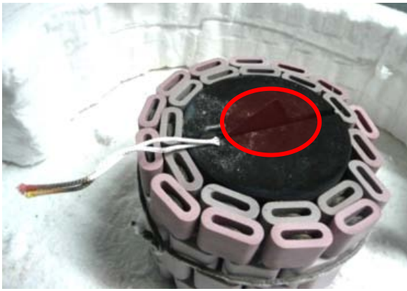
Fig. 3 : Photograph of larger mass holder covered with heater, part marked as red circle
