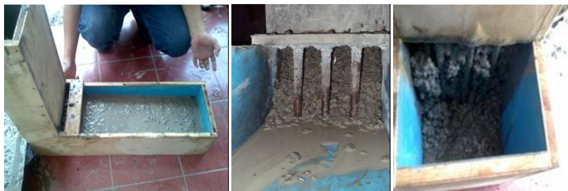
(a) SCC with 1% fine tire fibre (b) blocking SCC 1% cans fibre (c) blocking on U-box test
