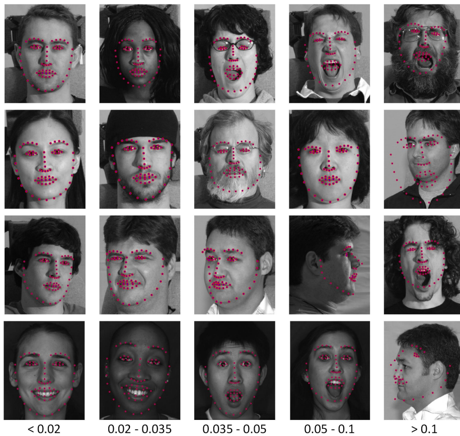
Figure 4.15: Comparing different RMS errors. Notice how the landmark detection can no longer reliably identify all of the regions of the face, with errors above 0.05.
