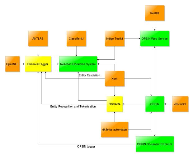
**Figure 2-17:** How the open source projects involved in this project relate to each other. Green projects are projects developed predominantly for this project whilst yellow projects are those in which significant improvements were undertaken. Utility and unit testing libraries are not shown.
