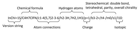
Figure 2-7 Standard InChI string with layers annotated
