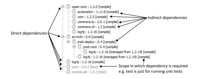
Figure 2-16 Dependency hierarchy for the opsin-inchi module
