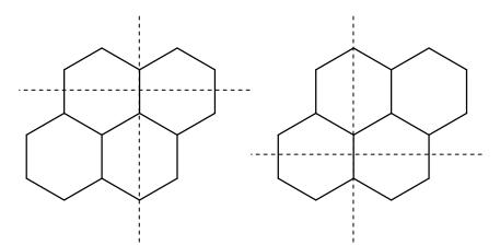
**Figure 3-87** Lines showing the quadrants for the two possible horizontal row candidates of this grid layout. The right interpretation is preferred as more rings are in the upper right quadrant.
