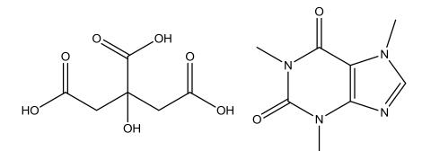
**Figure 3-121** caffeine citrate. Citrate in isolation would be treated as a tri anion but as there is another compound present it is treated as if it were citric acid.
