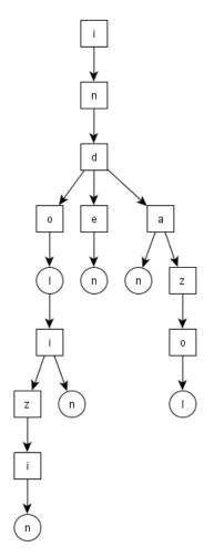
**Figure 3-7** A trie describing indol, indolizin, indolin, inden, indazol and indan. Circular nodes are accepting nodes
