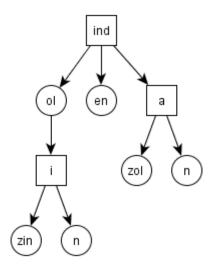
**Figure 3-8** A radix trie describing indol, indolizin, indolin, inden, indazol and indan. Circular nodes are accepting nodes
