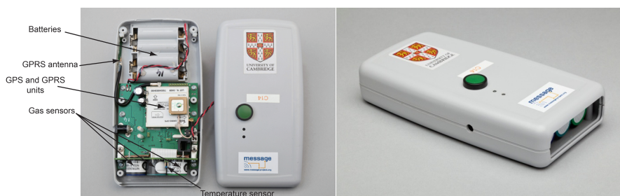
Figure 3.1. Mobile sensor unit incorporating three electrochemical sensors (for CO, NO and NO 2 in this case). Various components (GPS/GPRS, batteries etc.) are identified in the left panel. For clarity, the unit is shown without its protective wire mesh, which, during operation, is located in front of the sensors.
