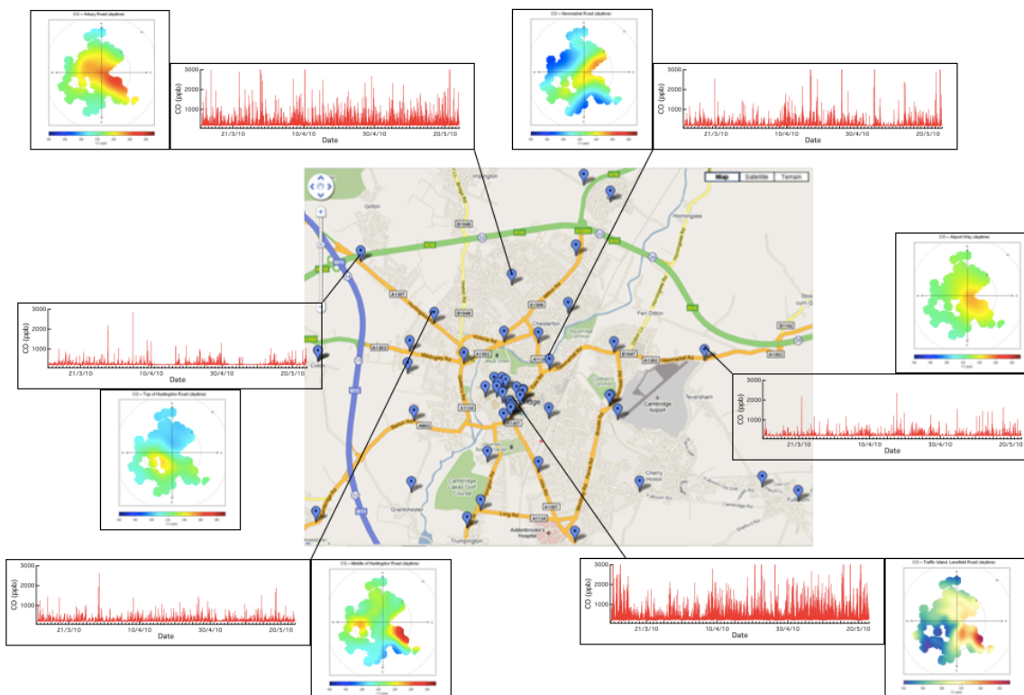
Figure 4.4. Selected time series and bivariate polar plots for daytime carbon monoxide measurements obtained during a 2.5-month deployment of lamppost-mounted sensor nodes, as described in section 4, in the Cambridge area, illustrating typical variability (see text for further discussion). Time series plots have identical ordinate scales. Bivariate plots are also on identical scales, with the exception of the central Cambridge site (bottom right) which, for clarity, has a different colour scale. Cambridge meteorological data is courtesy of the University of Cambridge Computer laboratory Digital Technology Group.
