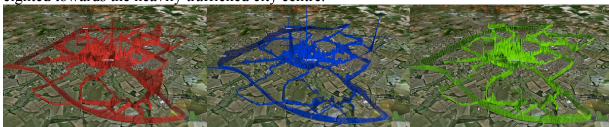
Figure 3.9. 3D plots (left to right respectively) of CO, NO and NO 2 mixing ratios giving overviews of measurements obtained during a large, mobile sensor deployment. The peak heights correspond to mixing ratio, with maximum values of 7 ppm, 4.5ppm and 840 ppb for CO, NO and NO 2 respectively (map data © 2012 Google and © 2012 Infoterra Ltd & Bluesky).
