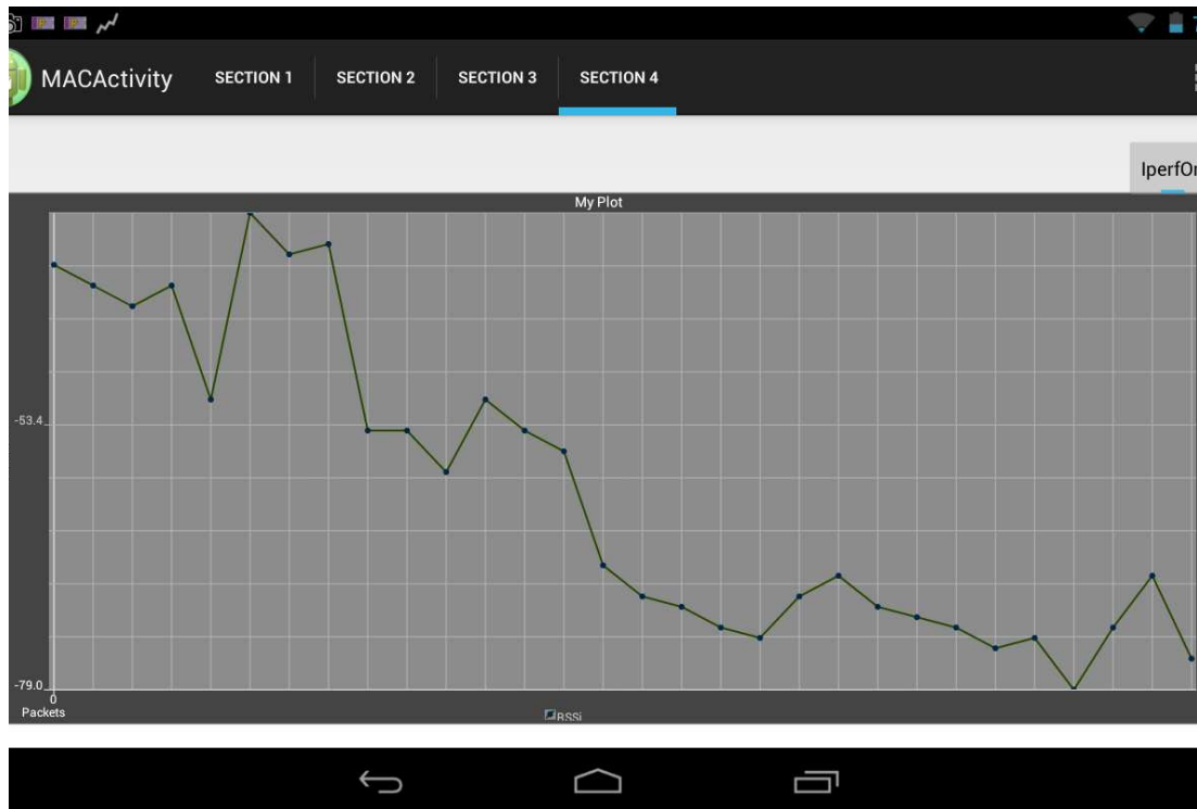
Figura 7.1: RSSi values of two nodes in dBm, each tick is approximately one second
