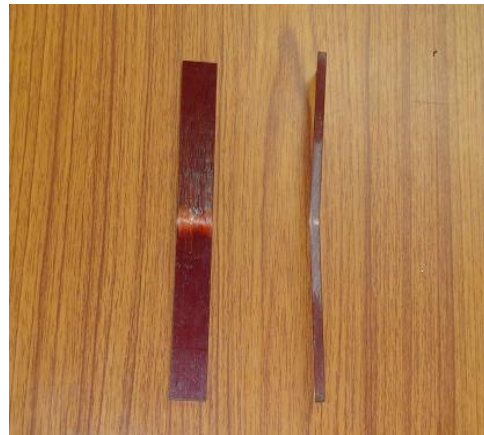
Figure 5. Typical flexural failure mode
