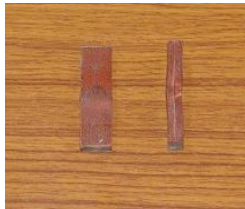
Figure 7. Typical ILSS failure mode
