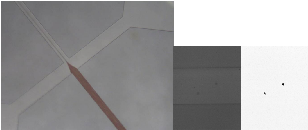
Figure 9. Hydrodynamic flow focusing in a microchannel using intravenous blood (left side image). Original high-fps image using 60us exposition time (center), processed image with only cell like objects (right side image).
