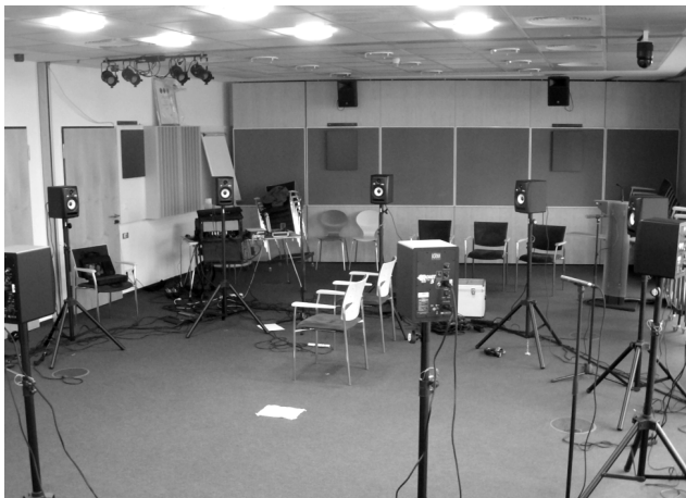
Figure 2: Photograph of the speaker setup in the measurement room.
