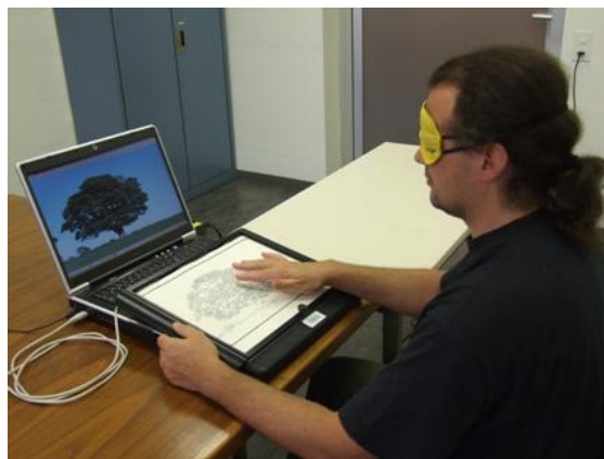
Figure 3: Example of an embossed picture on the T3 tactile tablet.
