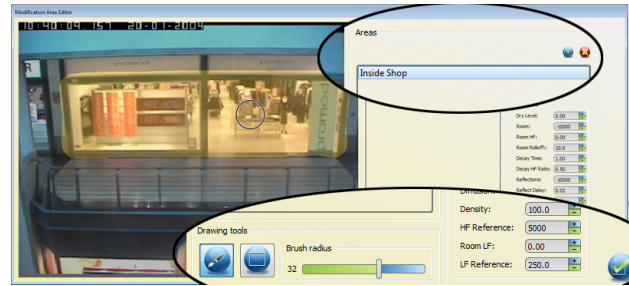
Figure 3: Graphical user interface for the definition of a modification area. Left: specification of the region of influence by Photoshop-like brushing (the circle shows the brush). Right: specification of modification filters and their parameters.
