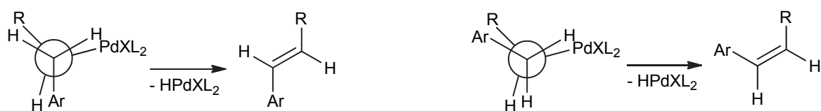
Figure 4 The eclipsed conformations prior to the \beta -hydride elimination leading to E or Z olefin
