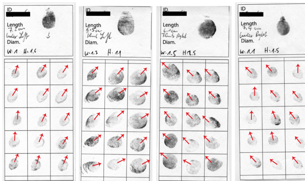
FIGURE 4.29: An example of the actual size of the finger and thumb of a user when touching the screen in 15 positions. From left to right: Left index finger, left thumb, right thumb, right index finger. To record the prints, a sheet of paper showing a grid combining four target positions of the application (Fig. 4.1, p. 132) into one square was attached to the phone's screen. Users pressed their fingers onto an ink pad and randomly tapped onto each square while holding the phone in the same way as they would when operating the application. Red arrows were superimposed to indicate the touch direction.
