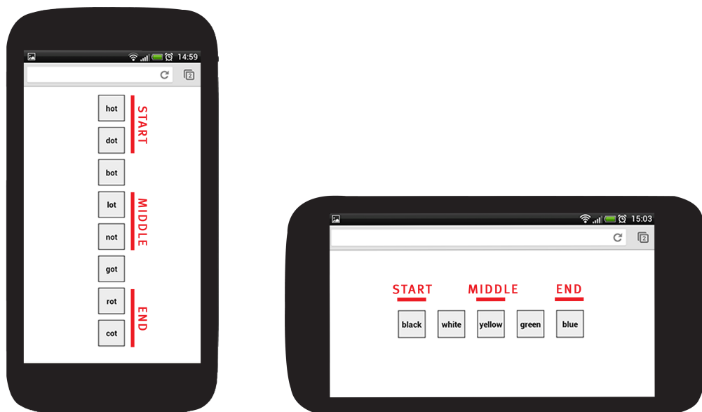
FIGURE 3.2: Left: A layout of eight buttons in portrait orientation in R1. Right: A layout of five buttons in landscape orientation in R2. The three target zones are superimposed in red. Images taken from Seipp and Devlin (2013 b ).
