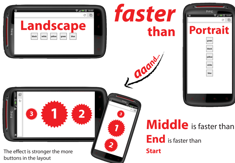
FIGURE 3.10: The observed efficiency ranking of the three target zones in R2. Middle is fastest, followed by End , followed by Start . This applies to landscape and portrait orientation. In addition, interaction with a device in landscape orientation is faster than in portrait orientation.
