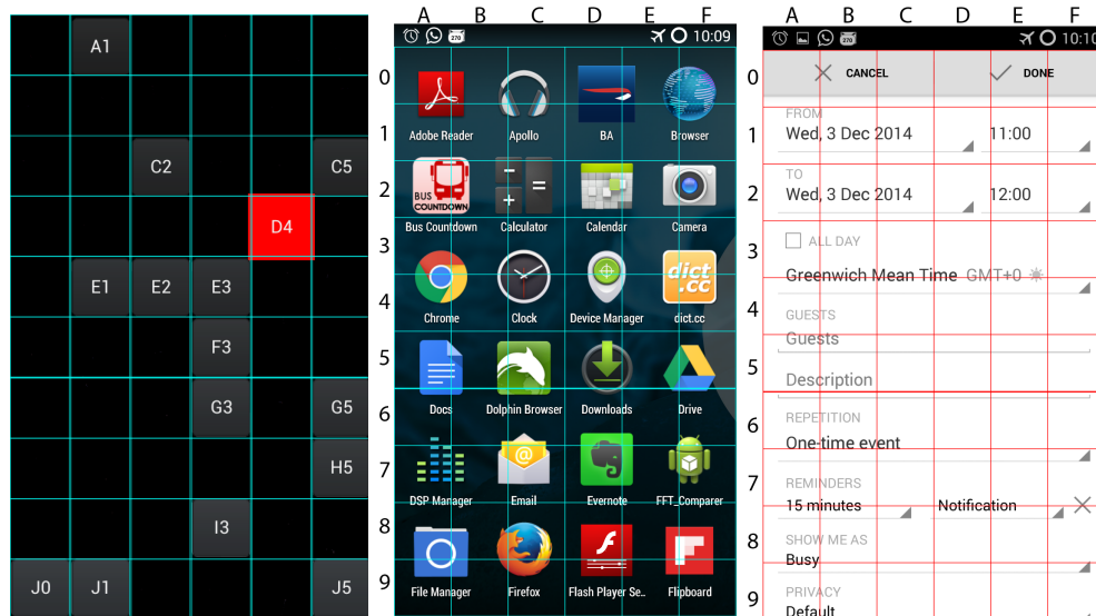
FIGURE 4.58: Left: The collection of the touch data for each of the 60 grid units. Buttons are located in each grid unit to facilitate collection. Middle: An invisible grid is laid over an application interface. Incoming touches are attributed to a grid unit and evaluated based on the previously collected data. Right: More complicated layouts could employ the technique, as hitting a unit off-centre is of little relevance due to the unimportance of the X Offset property for finger classification.
