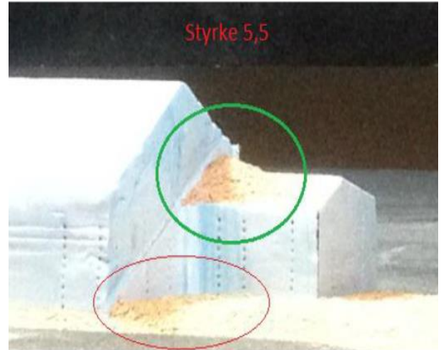
Figure 11: Model of the snow accumulation in Greenland referring to real life observations. Airspeed and material are adjusted to reflect the snow drift mechanism at reduced model scale in the wind tunnel study.
