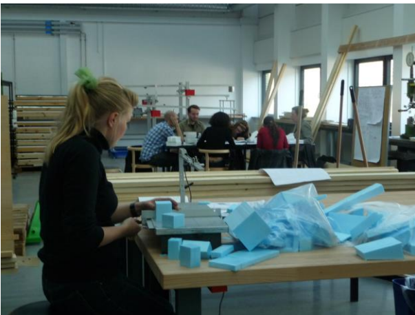
Figure 2: Shaping the models for the tunnels in foam by means of a hot-wire cutter.
