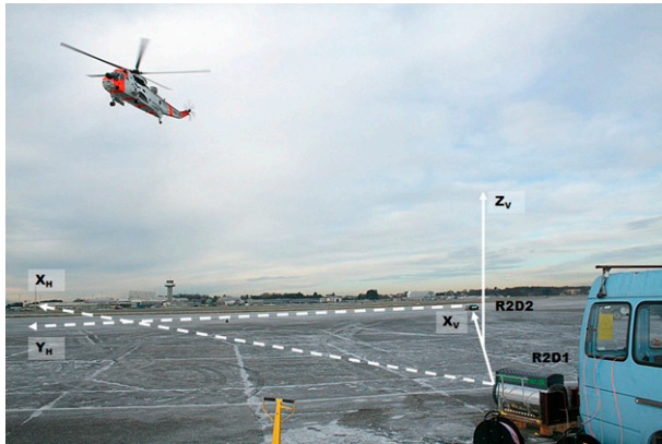
FIG. 1. The image shows the experimental setup for scanning a horizontal plane beneath the hovering helicopter. Note that for scanning the vertical plane, the helicopter was instead hovering above the center of the line between the R2D1 and R2D2 WindScanners. The coordinate system used for the horizontal scan is outlined by dashed lines and index H, whereas the coordinate system used for the vertical scan is outlined by solid lines and index V.
