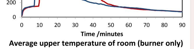
those noted in the PIR room. The average temperature in the upper layer compartment was lower overall despite longer burner time at 600 kW and increased test duration (left).
