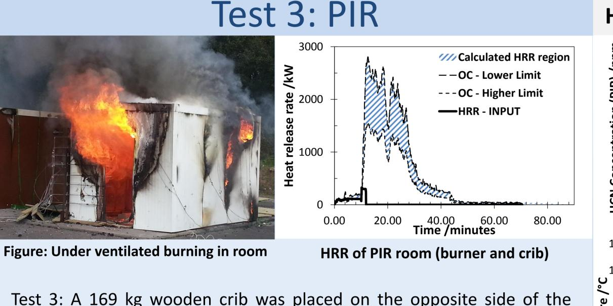
Test 3: A 169 kg wooden crib was placed on the opposite side of the enclosure, in addition to the burner. The crib ignited after 11 minutes (1 minute after stepping the burner up to 300 kW) from radiation above, and took 2 minutes for the flames to reach the bottom of the crib.
