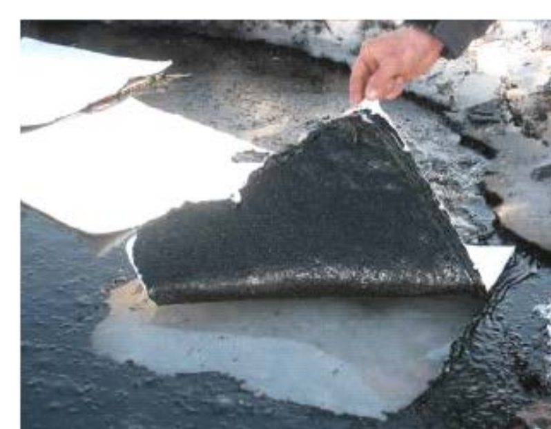
Manual cleaning of oil. Effective but unpractical (Photo: P. J. Brandvik)
