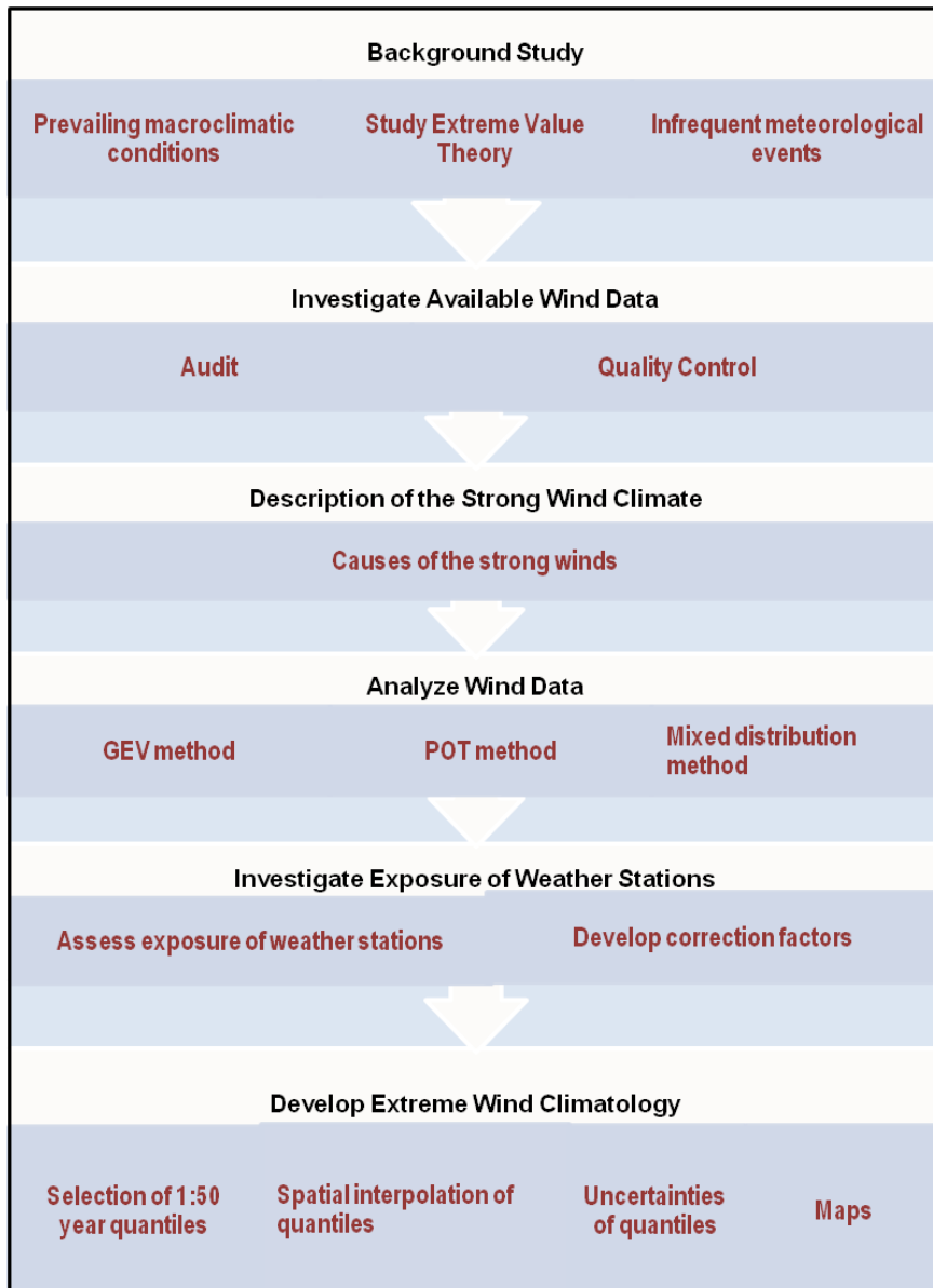
Figure 4. Optimal procedure for the estimation of design wind speeds from measured data (Kruger 2010).
