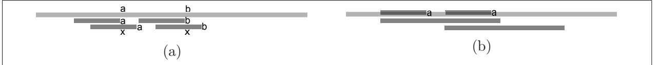
Figure 3: The new string-matching algorithm using slubs: (a) sparsify to one candidate in each |z| + 1 block: after verifying the size 2 deterministic sample \{a, b\} , any surviving occurrence candidate that has another close-by candidate on its left, can be eliminated. (b) sparsify to one candidate in each period length \pi(x) block: after verifying the deterministic sample za , any surviving occurrence candidate that has another close-by candidate on its right, can be eliminated.
