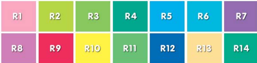
Figure 2.13. Test colors used for CRI calculations.
