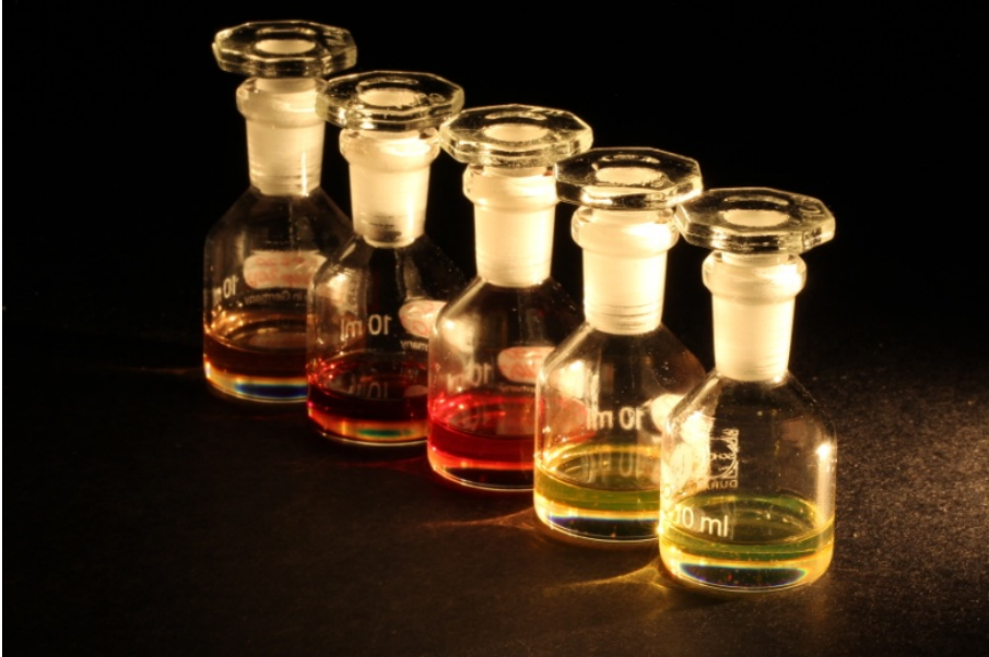
Figure 2.10. Example of different emission wavelengths CdSe/ZnS colloidal QDs in solution.
