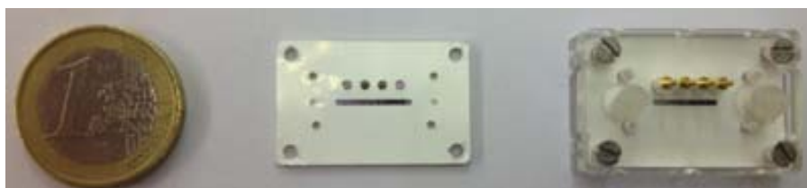
Figure 43. PPF microband flow cell to detect mercury in water samples.
