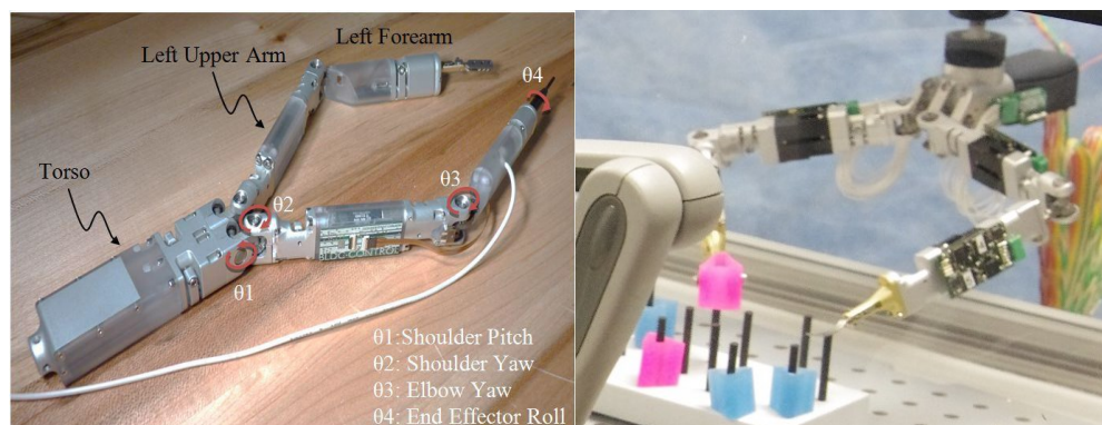
Figure 4.2. EricBot 2.0 (left) and EricBot 2.1 (right) Note: EB2.0 is not shown with wiring between joints.
