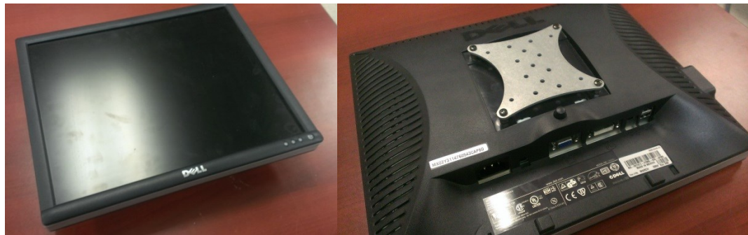
Figure 4.5. Dell monitor with custom mounting plate attached
