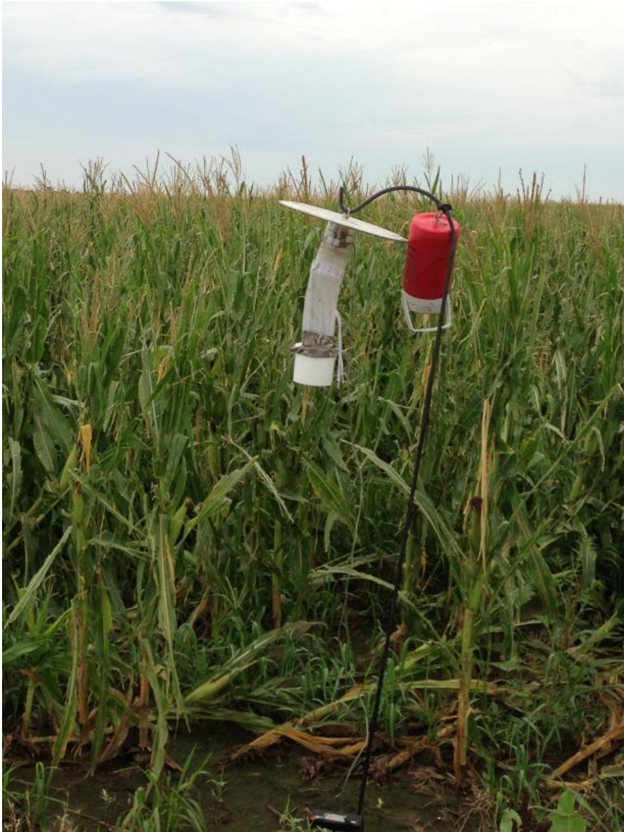
Figure 2.4 CO 2 -baited CDC miniature light trap assembly
