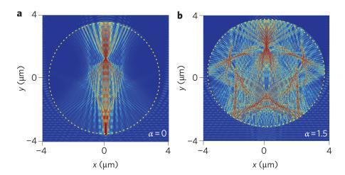
Figure 6.13: Ab-initio simulation results: snapshot of the electromagnetic energy density H distribution after t=45 fs in a resonator (dashed line) with  $V=30\mu m^2$  for  $\alpha=0$  (a) and  $\alpha=1.5$  (b).
