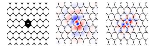
Figure 6.4: (*left*) Example of a point defect inside a PC lattice. Here it exhibits as a modification of the radius of a single column that composes the lattice. Electric (*centre*) and magnetic (*right*) fields inside the defect. Colours represents the intensity of the field that is localized inside the defect.
