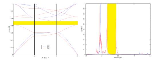
Figure 6.18: Band diagram of the triangular lattice constituted by silicon ( $\varepsilon = 12$ ) with air columns of radius r = 0.46a obtained with different programs: MPB (*left*) and NANOCPP (*right*). Results are in good agreement showing a complete band gap in the range  $\lambda = [2.17, 2.44]a$ .
