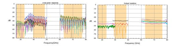
Figure 1.11: Side arm cross-polar response (left) and output isolation (right) for all the eleven OMT (amplitude). the LFI frequency bands are evidenced in the figure [55].
