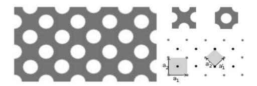
Figure 6.1: (*left*) Example of a 2D triangular lattice. (*right*) Examples of unit cells and primitive translation vectors that can be identified inside this lattice.
