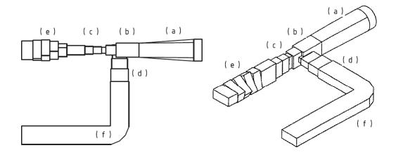
Figure 1.10: Sketch of the 44 GHz OMT used in the LFI *Planck* instrument [55].
