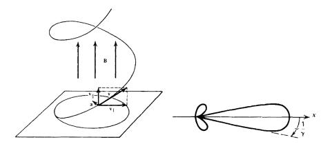
Figure 2.8: Left. The helical motion of a charged particle in an uniform magnetic field. Right. The angular distribution of the radiation emitted. The arrow is perpendicular to the acceleration and tangent to the circular motion [135].
