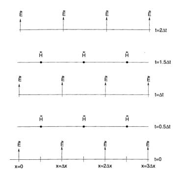
Figure 6.7: Space-time grid of the Yee algorithm for a one-dimensional case. This grid definition allows the use of central differences for the space derivatives and leapfrog for the time derivatives.
