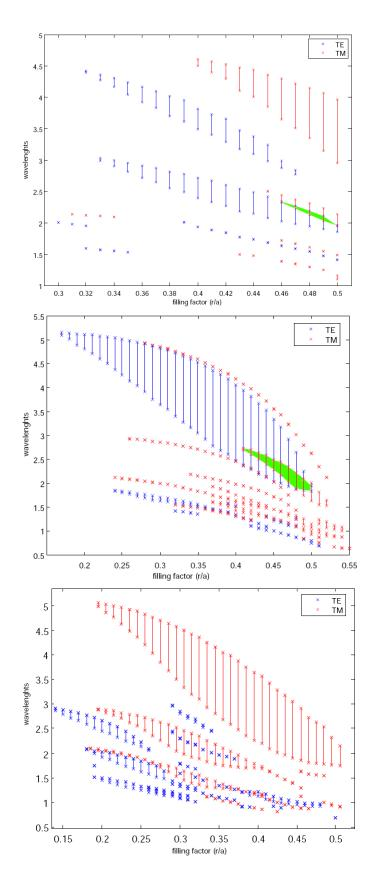
Figure 6.17: The extensions of the photonic band gaps for TE and TM modes (respectively blue and red lines) versus the filling factor (r/a) for different lattices: square (top panel), triangular (center panel) and honeycomb (bottom panel). For all the cases the PC are constituted of holes of radius r inside a slab of silicon ( $\varepsilon \simeq 12$ ).
