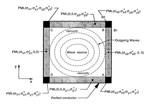
Figure 6.10: Structure of a two-dimensional FDTD grid with at the boundaries the PML absorbing conditions.
