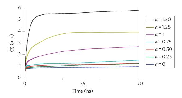
Figure 6.14: Time evolution of the average electromagnetic energy  $\langle E \rangle$  inside cavity resonators for different values of  $\alpha$ .
