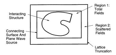
Figure 6.8: Subdivision of the computational region. The total field is present in region 1, while only the scattered field can propagate in region 2. On the connecting surface the algorithm is modified to keep the consistency of the equations.
