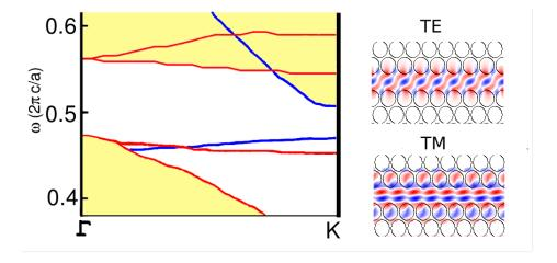
Figure 6.6: (*left*) Band diagram of a triangular lattice with a linear defect. White region that indicates the frequencies that cannot propagate in the crystal. The red and blue lines inside the white region describe respectively the TE and TM modes propagating inside the waveguide. (*right*) TE modes (*top*) and TM modes (*bottom*) propagating inside the waveguide built in a triangular lattice.
