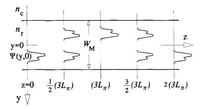
Figure 6.12: Schematic illustration of multimode waveguide showing the input field profile and a mirrored single image at  $(3L_{\pi})$ , a direct single image at  $2(3L_{\pi})$ . and two-fold images at  $\frac{1}{2}(3L_{\pi})$  and  $\frac{3}{2}(3L_{\pi})$  [300].
