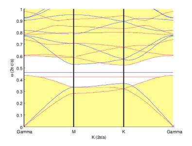
Figure 6.5: Band diagram of a triangular lattice with a point defect shown in Fig. 6.4. White regions represent the band gap, that is the frequencies that cannot propagate inside the crystal. The two horizontal lines describe the TM mode (red) and TE mode (TE) that can be excited in a localized field inside the cavity.
