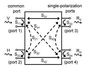
Figure 1.9: Representation of an OMT with relevant port-signals [56].
