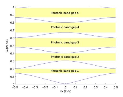
Figure 6.3: Band diagram for a 1D PC in which the unit cell is composed by two layers alternatively of air ( $\varepsilon = 1$ ) and silicon ( $\varepsilon = 12$ ). There are 5 different photonic band gaps.
