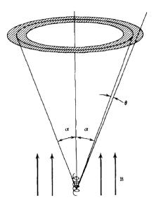
Figure 2.9: Synchrotron emission from a particle with pitch angle  $\alpha$ . Radiation is confined to the shaded solid angle [135].
