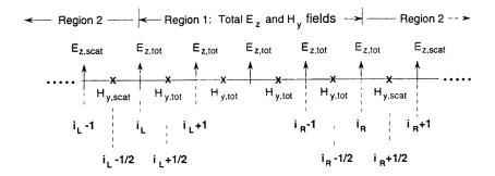
Figure 6.9: One dimensional example of the spatial disposition of the points and of the electric and magnetic fields. The two regions are described at the top. It is evident the inconsistency of the fields along the connecting surface.
