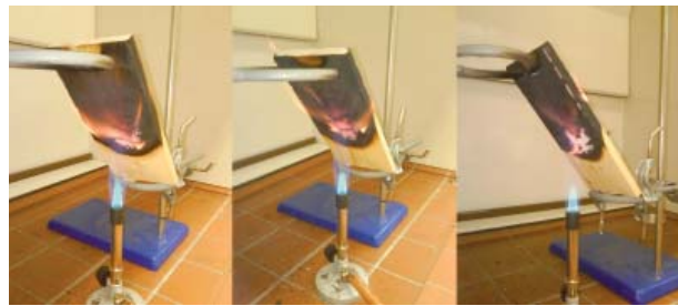
Fig. 2 The simulation of testing of fire retardant Plamostop Standard
