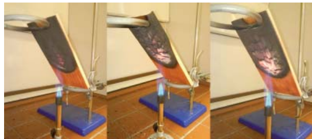
Fig. 3 The simulation of testing of fire retardant Falured - Nanopol
