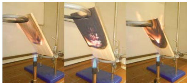
Fig. 4 The simulation of testing of fire retardant Cloisite
