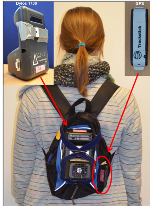
Figure 3-4 The monitoring pack - the Dylos monitor is strapped onto the backpack with the inlet and fan exposed to the air. The GPS is placed in the side mesh bottle pocket.
