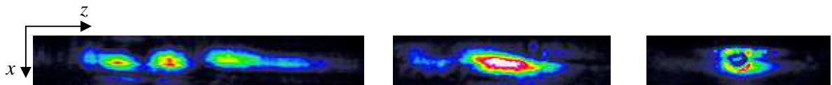
Figure 4.6: Images of group A, written in titanium waveguide. a) A1 guide, characterized by a multi-mode propagation of light. b) A2 guide, where the propagation is mono-mode. c) A3 guide, with a mono-mode propagation, in which a defect owed to the crystal is present.
