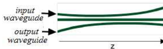
Figure 1.11: Waveguide structure providing an optical analogies to the intuitive three state STIRAP process.
