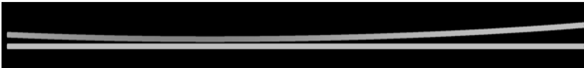
Figure 3.9: Image used to reproduce with the SLM in the SBN the desired pulse configuration. The present structure corresponds to the one for the counterintuitive case is reported.
