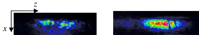
Figure 4.8: Images of group D, wrote in titanium waveguide. a) D1 guide, created in a crystal defect. b) D2 guide, where the propagation is mono-mode, and where a defect owed to the crystal is present.
